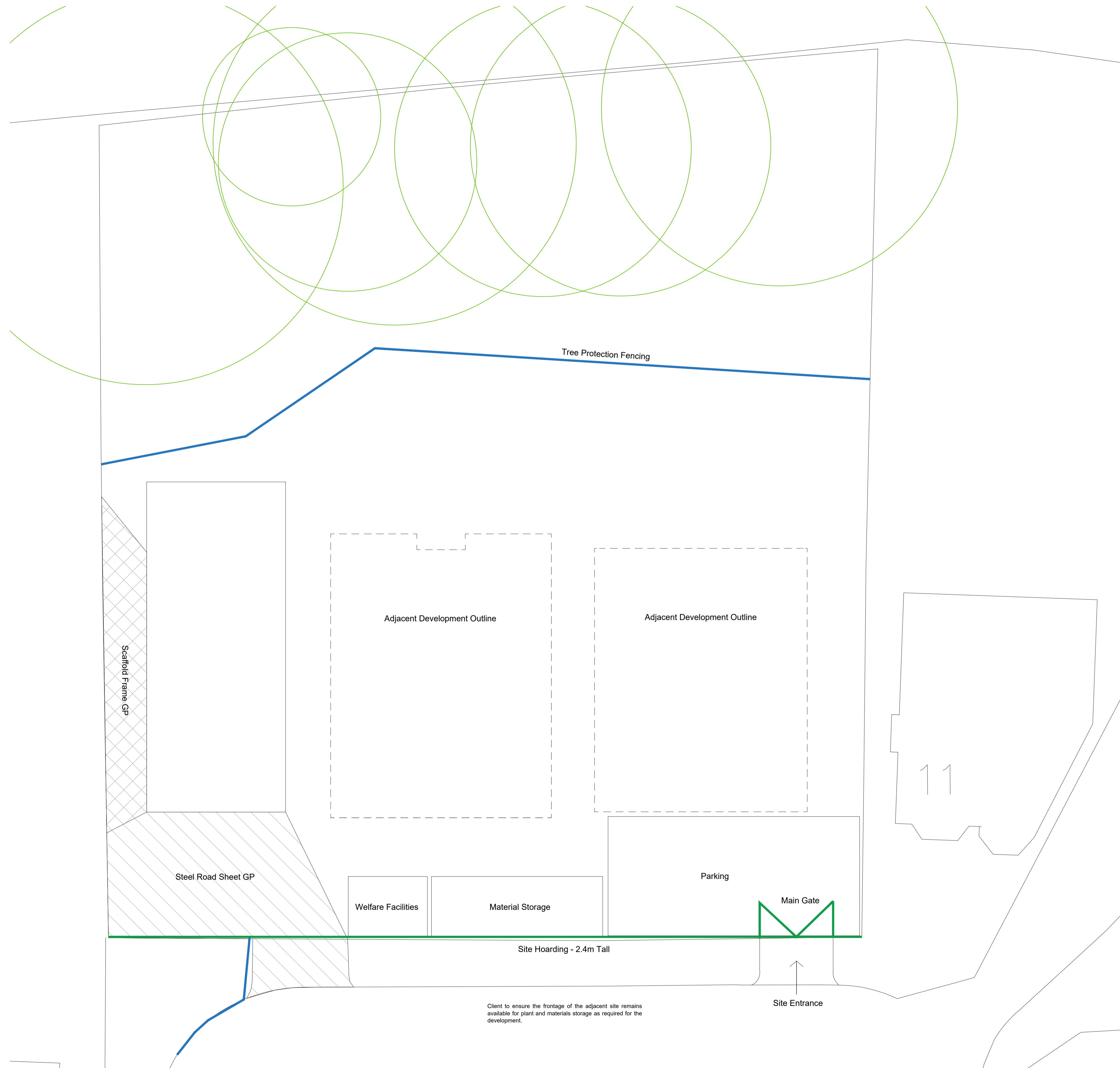
PROPOSED SITE LAYOUT DURING CONSTRUCTION - 1:100
